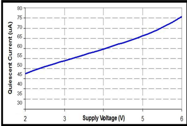
Quiescent Supply Current vs. Supply Voltage
