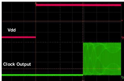
Figure 17. Startup Waveform vs. Vdd
