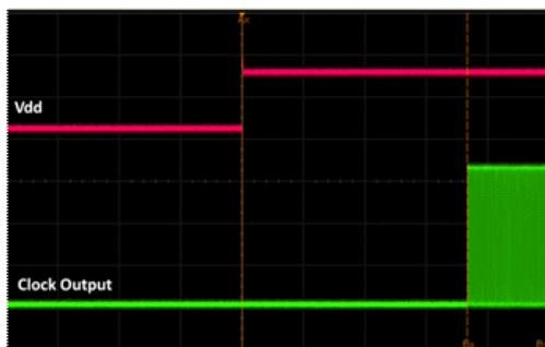
Figure 17. Startup Waveform vs. Vdd
