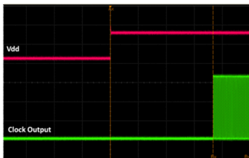
Figure 17. Startup Waveform vs. Vdd
