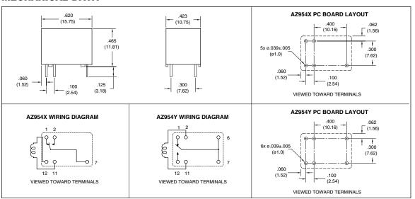
Dimensions in inches with metric equivalents in parentheses. Tolerance: ±0.010"
