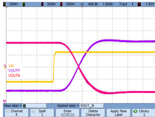
Figure 50. Step Response of the AMC1301 Device
