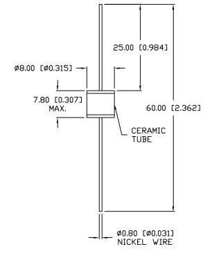
\*TOLERANCES PER DECIMAL PRECISION ARE: X=±1 (±0.039), X.X=±0.5 (±0.020), X.XX=±0.25 (±0.010), X.XXX=±0.127 (±0.005). LEAD LENGTH=±0.75 (±0.030). MIN= +DECIMAL PRECISION MAX.= +0.00 -DECIMAL PRECISION MAX.= +0.00 -DECI
