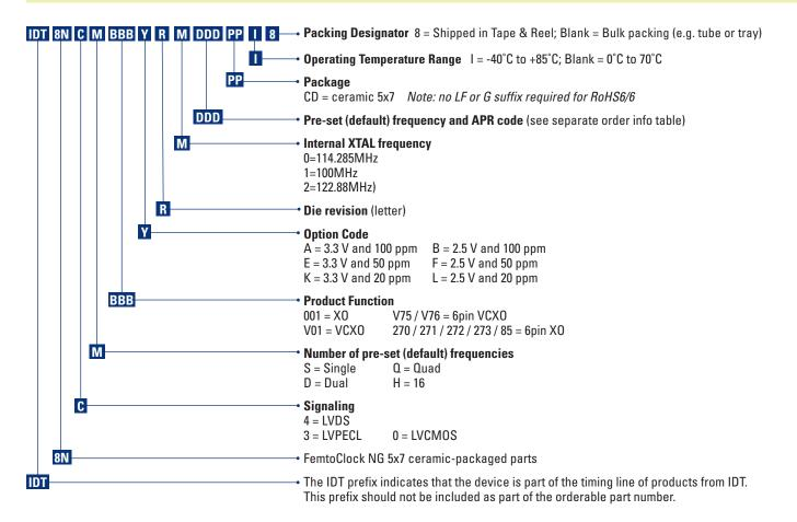
Example: IDT 8N3Q001LG-0001CDI8 is a LVPECL FemtoClockNG programmable oscillator, quad output frequency (125, 100, 122.88, 156.25 MHz), 2.5 V, 20 ppm, G-revision, 114.285 MHz XTAL in a RoHS 6/6 ceramic 5x7 package with tape and reel.
