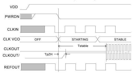
CLKIN must have a stable clock input when PWRDN is de-asserted. If CLKIN starts after PWRDN is de-asserted then Tstable specification applies to when CLKIN is ON. If CLKIN is full ON before PWRDN is de-asserted then the Tstable specification applies.
