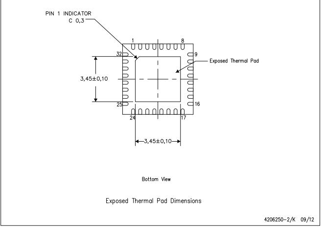
NOTE: All linear dimensions are in millimeters
