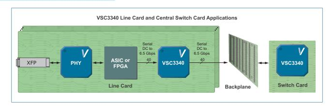
Using the VSC3340 in high-speed line cards ensures best-in-class I/O performance up to 6.5 Gbps with EQ technology to compensate for connector, backplane, and FR-4 loss. The VSC3340's small 23 mm  $\times$  23 mm form factor enables use in line card or central switch applications.
