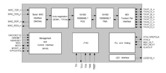
The VSC8634 is a low-power quad Gigabit Ethernet transceiver ideal for high-density switch and router applications. The device's compact package is optimal for multiport switch applications. Vitesse's mixed signal and DSP architecture yield robust performance, supporting both full and half duplex 10BASE-T, 100BASE-TX, and 1000BASE-T over >140 meters of Cat5, unshielded twisted pair cable, with industry leading tolerance to NEXT, FEXT, Echo, and system noise.
