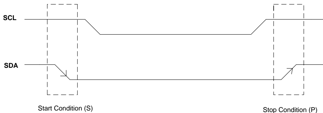
Figure 1. I 2 C Start and Stop Condition
