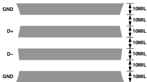
Figure 8. Arrangement of Signal Tracks
