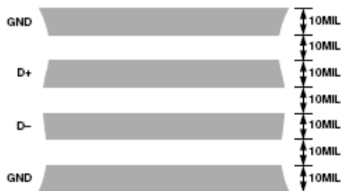
Figure 16. Arrangement of Signal Tracks
