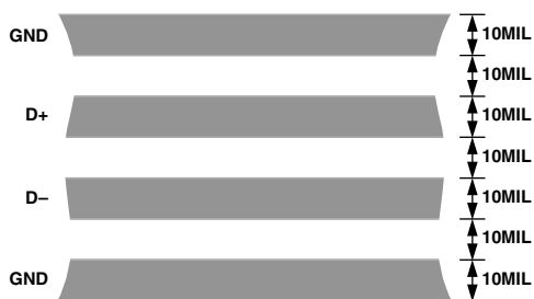
Figure 8. Arrangement of Signal Tracks
