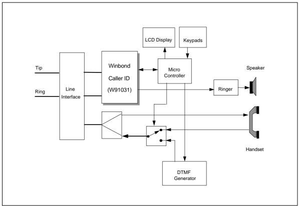
Figure 5. System Diagram for Caller ID Application
