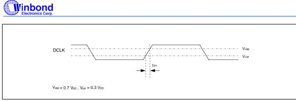
Figure 8-7. DCLK Mode 1 Input Timing
