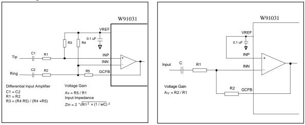
Figure 7-2 Differential Input Gain Control Circuit
