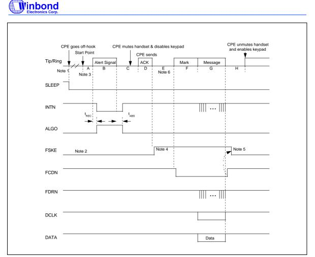
Figure 9-6. Input and Output Timing of BT Loop State (Off-hook) Data Transmission
