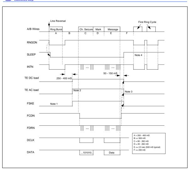
Figure 9-7. Input and Output Timing of CCA Caller Display Service Data Transmission
