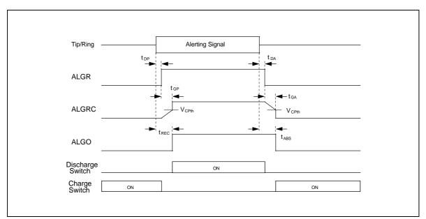
Figure 7-5. Guard Time Waveform of ALGR, ALGRC and ALGO Pins
