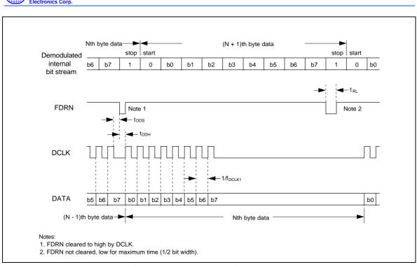
Figure 7-8. Serial Data Interface Timing of FSK Demodulation in Mode 1
