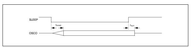
Figure 8-1. Wake up and Sleep Down Timing
