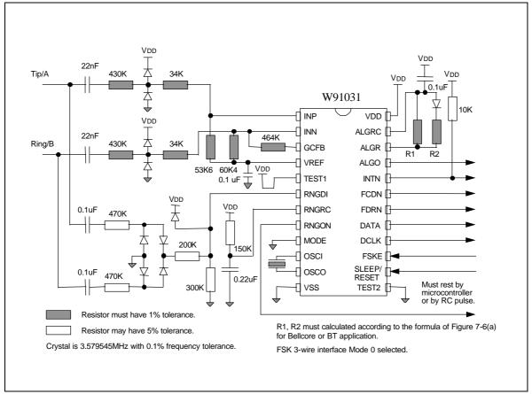
Figure 9-1. Application Circuit.
