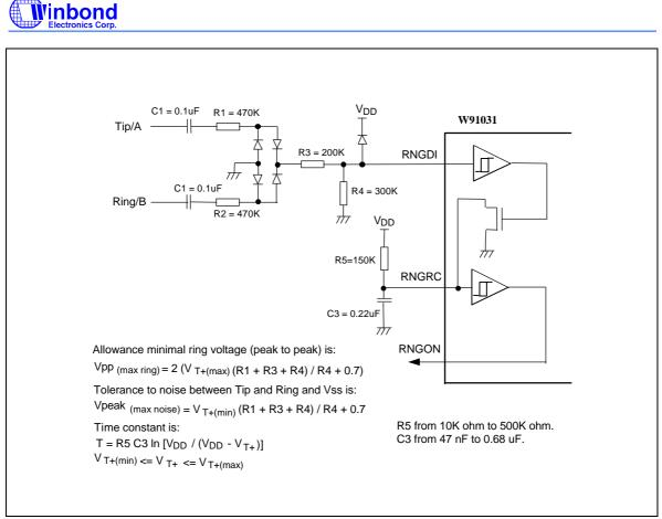
Figure 7-1. Application Circuit of the Ring Detecter
