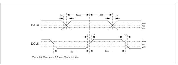
Figure 8-4. Data and DCLK Mode 0 Ouput Timing
