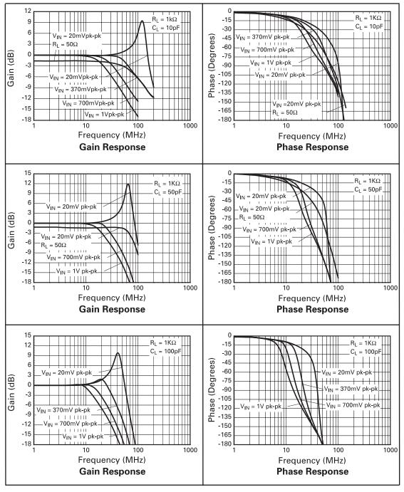
Test Conditions:V+=5V, Temperature=25°C.
