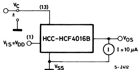
SWITCH THRESHOLD VOLTAGE IS DEFINED AS THE VOLTAGE APPLIED TO A TRANSMISSION GATE CONTROL WHICH CAUSES  $10\mu\text{A}$  OF TRANSMISSION GATE CURRENT.
