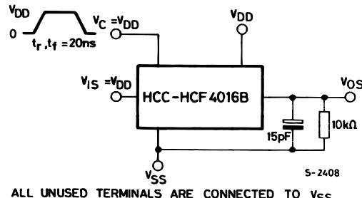
PROPAGATION DELAY TIME SIGNAL INPUT ( $V_{IS}$ ) TO SIGNAL OUTPUT ( $V_{OS}$ )
