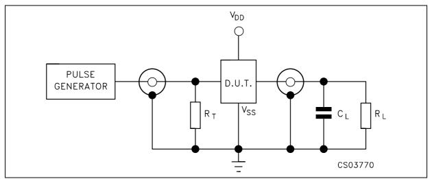
$C_L$  = 50pF or equivalent (includes jig and probe capacitance)  $R_L$  = 200KΩ  $R_T$  =  $Z_{OUT}$  of pulse generator (typically 50Ω)
