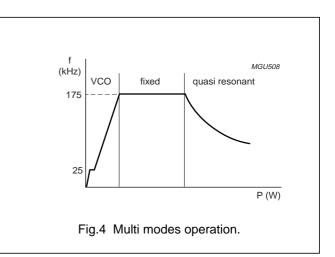
The next converter stroke is started only after demagnetization of the transformer current (zero current switching), while the drain voltage has reached the lowest voltage to prevent switching losses (green function). The primary resonant circuit of the primary inductance and drain capacitor ensures this quasi-resonant operation. The design can be optimized in such a way that zero voltage switching can be reached over almost the universal mains range.
