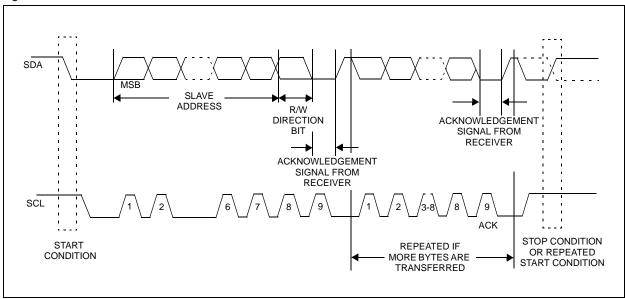
Figure 25. Data Transfer on I<sup>2</sup>C Serial Bus
