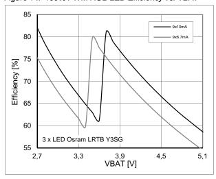
Figure 15. 100% PWM WLED Efficiency vs. VBAT
