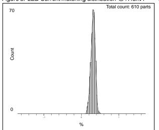
Figure 9. LED current Accuracy distribution @17.5mA
