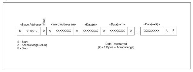
Figure 27. Data Read (Write Pointer, Then Read) - Slave Receive and Transmit
