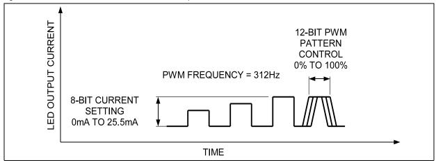
LED dimming is controlled according to a logarithmic or linear scale(see Figure 24). Logarithmic or linear scheme can be set for both the program execution engine control and direct PWM control.
