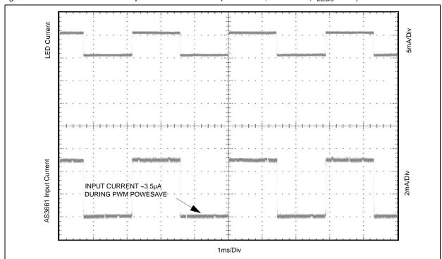
Figure 22. PWM Powersave Principle with external clock (VDD =3.6V, 50% PWM, I<sub>I FDQ</sub>=5mA)
