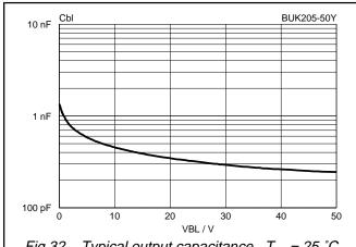
Fig.32. Typical output capacitance.  $T_{mb} = 25 \, ^{\circ}\text{C}$  $C_{bl} = f(V_{BL});$  conditions  $f = 1 \, \text{MHz}, \, V_{lG} = 0 \, \text{V}$
