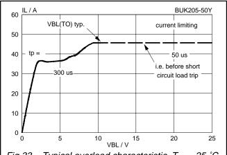
Fig.33. Typical overload characteristic,  $T_{mb} = 25$  °C.  $I_L = f(V_{BL})$ ; condition  $V_{BG} = 13$  V; parameter  $t_p$
