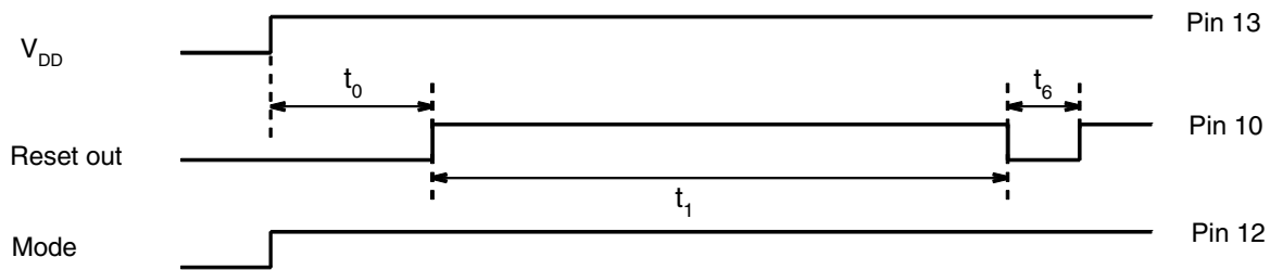
Figure 4-2. Power-up Reset and Mode Switchover
