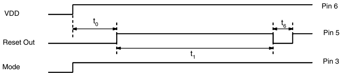
Figure 4-2. Power-on Reset and Switch-over Mode
