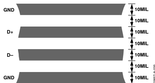
Figure 35. Arrangement of Signal Tracks
