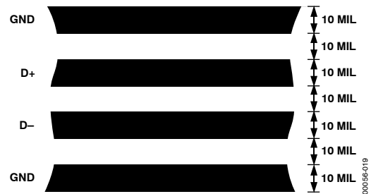
Figure 19. Arrangement of Signal Tracks
