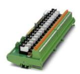
16-channel relay module for Honeywell C300 input modules. The module is controlled by the control system via 37-pos. D-SUB or 50-pos. FLK. A screw connection with knife disconnection is available in the field. Module width: 343 mm
