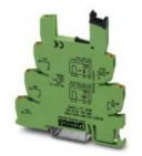
6.2 mm PLC basic terminal block for input functions with push-in connection, without relay or solid-state relay, for mounting on DIN rail NS 35/7,5, with sensor supply voltage distribution (BB), 1 N/O contact, input voltage 230 V AC/DC
