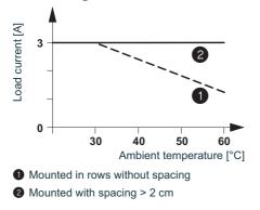
Figure 1 Derating curve for basic terminal block with power solid-state relay OPT- 5DC/24DC/2
