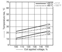
5-(2). Coil temperature rise Tested sample: TX2-48V, 6 pcs. Point measured: Inside the coil
