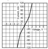
9. Off state leakage current
