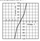
9. Off state leakage current
