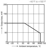
2. Relative output current vs. ambient temperature characteristics
