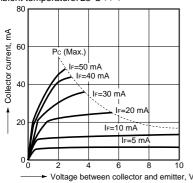
4-2. Collector current vs. voltage between collector and emitter characteristics (Ic-VcE)
