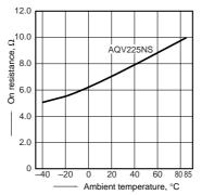
2.-(2) On resistance vs. ambient temperature characteristics
