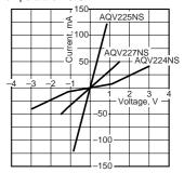
9. Off state leakage current
