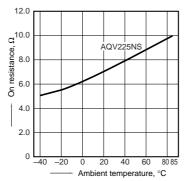
2.-(2) On resistance vs. ambient temperature characteristics
