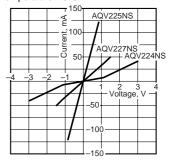
9. Off state leakage current
