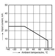
2. Load current vs. ambient temperature char-
