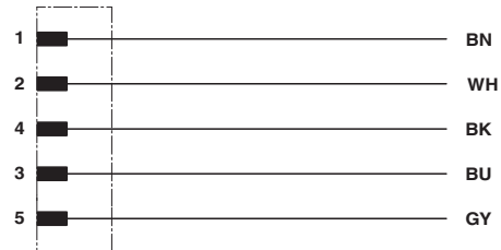
Contact assignment of the M12 connector
