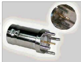
The press-fit center pin locks the connector into the PC board so it is held firmly for reflow or wave soldering.
