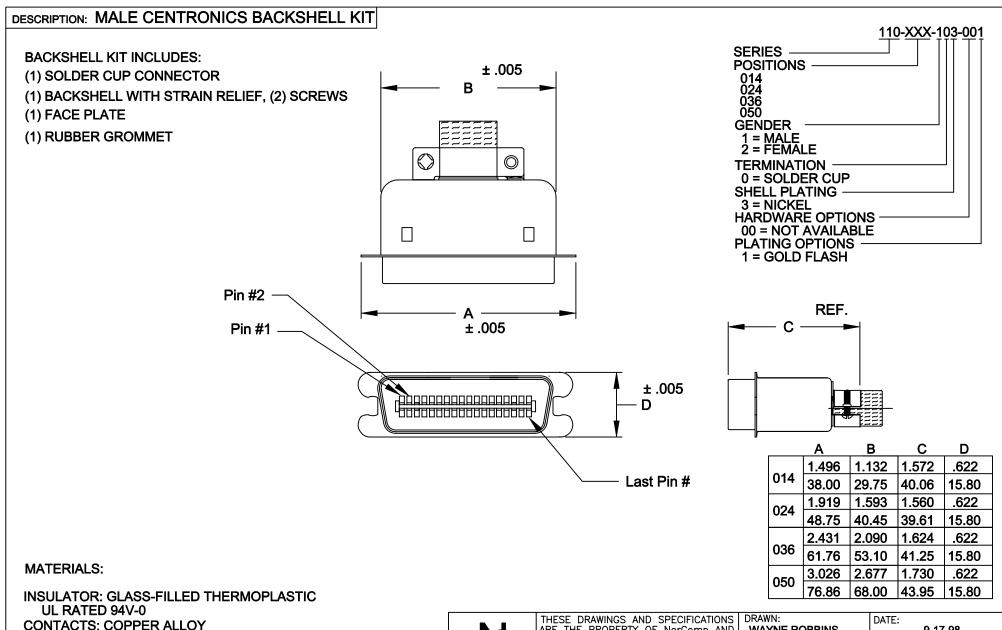
**CONTACT CURRENT RATING: 5 AMPS** DIELECTRIC WITHSTANDING VOLTAGE: AC 1200 R.M.S. INSULATION RESISTANCE: 1000 mohms MINIMUM AT 500V DC CONTACT RESISTANCE: 30 mOHMS MAXIMUM OPERATING TEMPERATURE: -55°C TO +125°C
