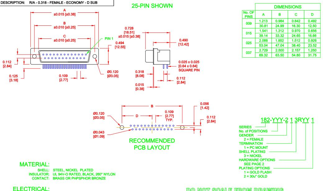
**CURRENT RATING: 5 AMPS** DIELECTRIC STRENGTH: 1,000VAC rms
