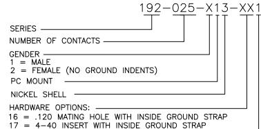
18 = 4-40 STANDOFF WITH INSIDE GROUND STRAP 53 = 4-40 INSERT WITH FORK BOARD LOCKS
