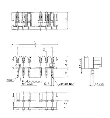
Note 1. The plug, which has the mark at the designated position, is for AWG26. Note 2. The cleaning by heat and trichloroethylene an't be implemented.
