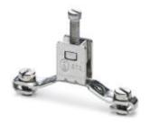
Ground modular terminal block, Connection method: Screw connection, Number of positions: 1, Cross section: 0.5 mm² - 16 mm², AWG: 20 - 6, Width: 8 mm, Color: silver, Mounting type: NS 35/7,5, NS 35/15
