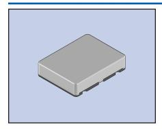
The VC-TXO-39SM is a VC (Voltage Controlled) TCXO (Temperature Compensated Crystal Oscillator) featuring very tight stability over a wide temperature range. The small SMD ceramic package measures  $11.4 \times 9.6 \times 2.3$  mm. The voltage control has a tuning range of  $\pm$  12 ppm typical. The low profile package is ideal for wireless communications applications.
