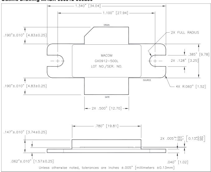
† Reference Application Note AN3025 for mounting/soldering recommendations. Meets JEDEC moisture sensitivity level 1 requirements. Plating is Ni/Au. Rev. V6
