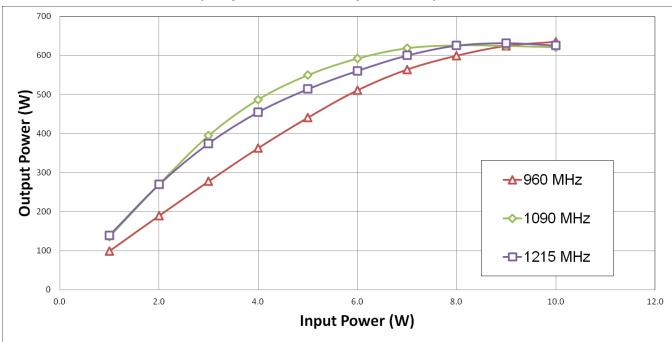
RF Power Transfer Curve (Output Power Vs. Input Power)
