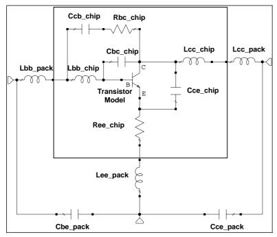
0.212 nΑ  $L_{\rm bb\_chip} =$ 0.07472  $L_{\rm cc\ chip} =$ nΗ 0.0184  $L_{\rm bb\_pack} =$ nΗ nΗ  $L_{\text{cc\_pack}} =$ 0.277 nΗ 0.239  $L_{\text{ee}\_\text{pack}} =$ 0.015 рF  $C_{\rm bc\ chip} =$ 0.013 pF  $C_{\text{cb\_chip}} =$ 0.282  $C_{\text{ce\_chip}} =$ pF 0.064 pF C<sub>be pack</sub> = 0.0492 pF  $C_{\text{ce}\_\text{pack}} =$ 7 Ω  $R_{\rm bc\ chip} =$ 0.566 Ω  $R_{\text{ee chip}} =$ Valid up to 6GHz
