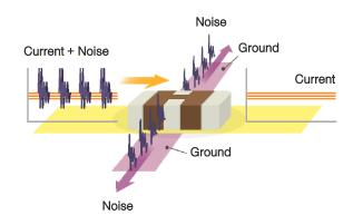
➤ When a pass-through structure is used, the smaller the distance between the capacitor and the ground, the lower the ESL. This helps reduce noise from the circuit.
