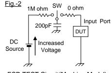
ESD TEST Circuit(Machine Model)
