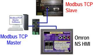
Shown above, the PC is the Modbus TCP Master and it is controlling/monitoring the remote slave (CP1H). The NS HMI communicates to the CP1H PLC via FINS. An Omron W4S Ethernet switch is used to connect the various Ethernet devices.
