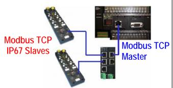
Shown above is a CP1H PLC with a CP1W-MODTCP01-US adapter configured for Master mode. It is communicating to two remote Omron IP67 Modbus TCP slaves. An Omron W4S Ethernet switch is used to connect the various Ethernet devices.
