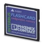
Program and configuration memory, plug-in, 2 Gbytes with license key for function block libraries, e.g., for: SNMP, SQL, wireless, motion functions, etc.
